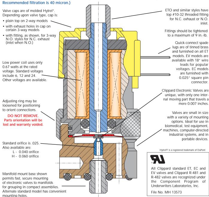
Clippard Minimatic electronic valves are precision-built 2-way or 3-way control valves, utilizing a unique, patented, valving principle. There are no sliding parts. Complete poppet travel is a mere 0.007". As a result, low power consumption and exceptionally long life are major benefits of this design.
